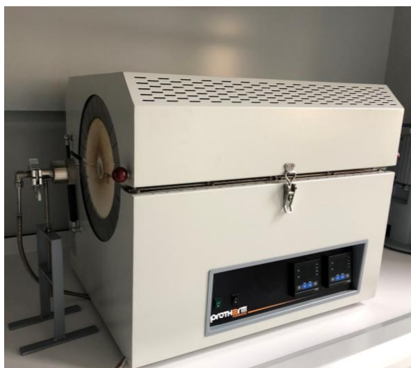
Figure 1. Annealing experimental setup (PROTHERM™ Furnaces).
