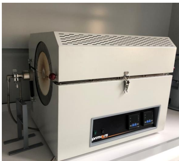
Figure 1. Annealing experimental setup (PROTHERM™ Furnaces).
